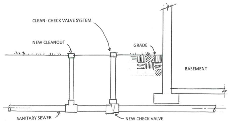
**Cautionary Note:** Check valves installed in sewer lines sometimes become clogged with debris and fail to close completely. When this happens, the valve will not stop the sewage completely. For this reason, a valve should not be depended upon completely, and the valve should always remain accessible for service and repair. Remember that when a check valve is installed in a house sewer, the house plumbing cannot be used during a storm when the valve is closed to prevent basement flooding.
